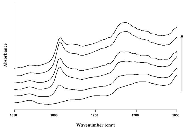
Fig. 4. Evolution of the FTIR spectra after several additions of \text{SnCl}_2 \cdot 2\text{H}_2\text{O} , TEMPO, MA. Each addition at the same concentration as the first one (0.04% (w/w) of \text{SnCl}_2 \cdot 2\text{H}_2\text{O} ; 0.04% (w/w) of TEMPO and 5% (w/w) of MA) was performed after 12 min: Catalyst first and 2 min later, TEMPO and MA. Sampling was performed just before each catalyst addition (12, 24, 36, 48 and 60 min after first MA feeding).
